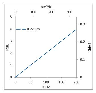
Flow rates for Cartridge filters are per 10-inch length. The test fluid is compressed air at ambient temperature.
