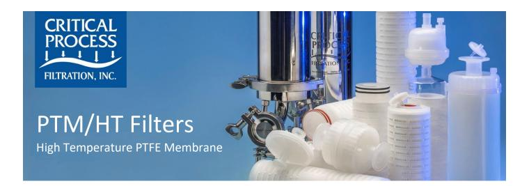
PTM/HT cartridge filters are made with Polytetrafluoroethylene (PTFE) membrane and high temperature polypropylene for cartridge hardware and membrane support. The filters are validated for sterilizing in elevated temperature gas and nonaqueous liquid applications (up to 221°F). Pore sizes range from 0.10 to 1.0 μm.
