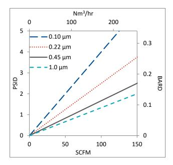
Flow rates for Cartridge filters are per 10-inch length. The test fluid is water or air at ambient temperature.
