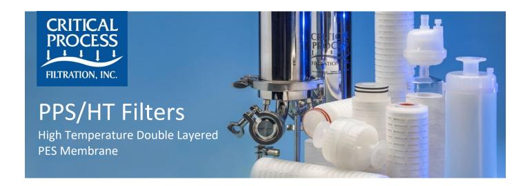
PPS/HT cartridge filters are constructed with a double layered Polyethersulfone (PES) membrane, high temperature polypropylene membrane support and high temperature cartridge hardware. They are for the critical sterilizing filtration of aqueous liquids. PPS/HT cartridge filters are validated for bacteria removal. Pore sizes range from 0.03 to 1.2  $\mu$ m.
